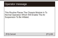
3) Carefully read the operation information on the screen, and press the operation step by step to select the [OK] to continue. Note that in some processes, the suspension height will change, and the engine should be turned off, and the power supply voltage is 12.5V.
