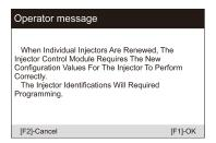
3) Follow the screen operation step by step, press the [OK] to perform the next step. In this process, the engine should be shut down, and the power supply voltage is 12.5V. Pay attention to the prompt of fuel injector code on the screen.
