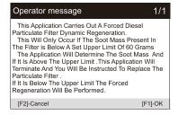
3) Follow the instructions on the screen step by step, and start the vehicle to drive at a speed higher than 40 km for about 15 minutes. Drive the vehicle to the required speed and press the "OK" button when the speed is reached.
