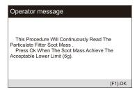
5) Regeneration is completed when it is indicated that the soot mass in the particulate filter is now at an acceptable lower limit. At this time, you can stop and turn off the ignition switch.
